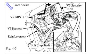
(g) Using the supplied bolt, secure the V5 security ECU and V5 GBS ECU to the reinforcement fixation. (Fig. 4-5)
