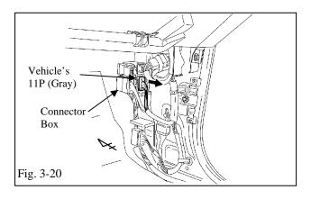
(y) Locate and disconnect the gray 11P connector to the connector block on the passenger side cowl area. (Fig. 3-20)
