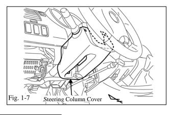
(m) Remove the lower steering column cover. (Fig. 1-7)
