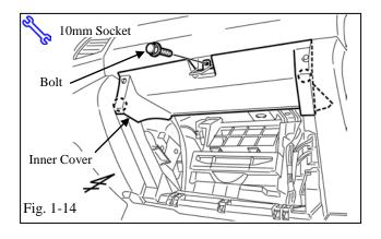
(v) Remove the glove box inner cover.
