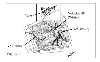
(v) Locate the vehicle harness' white 4P female connector and remove the tape securing the 4P connector. (Fig. 3-17)
