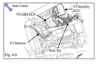
(h) Secure the V5 ECU harness and the GBS ECU portion of the V5 harness to the vehicle harness with one large wire tie. (Fig. 4-6)
