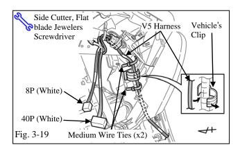
(x) Route and secure the V5 harness to the vehicle harness with two medium wire ties and the vehicle's wire clip. (Fig. 3-19)
